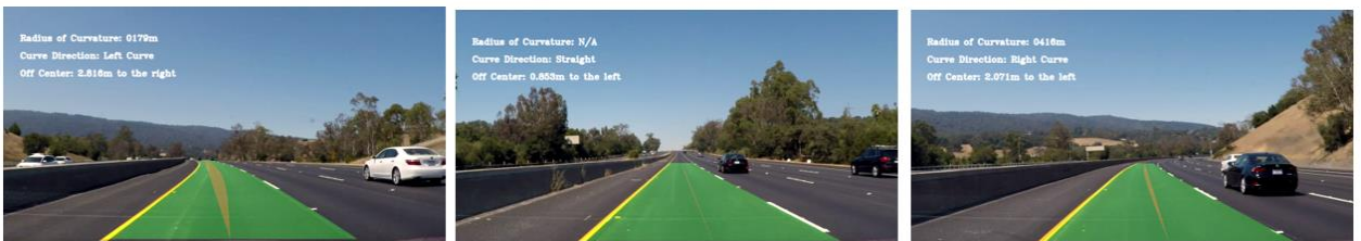
Fig. 6. Curvature estimation and directional analysis
