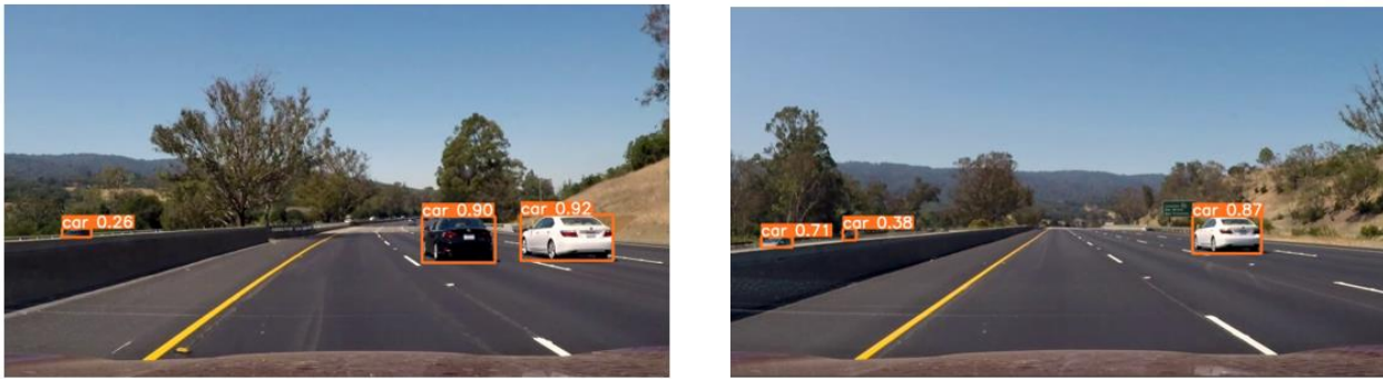
Fig. 7. Vehicle detection using YOLO
