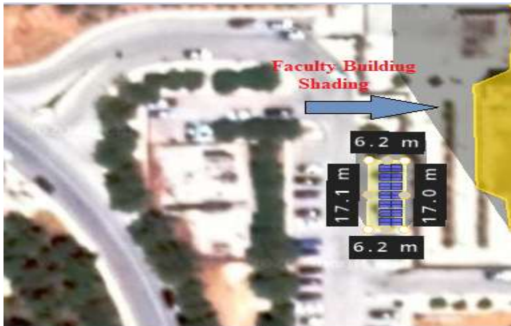
Figure 3.31 Location Area and Shading Via Helioscope Software
