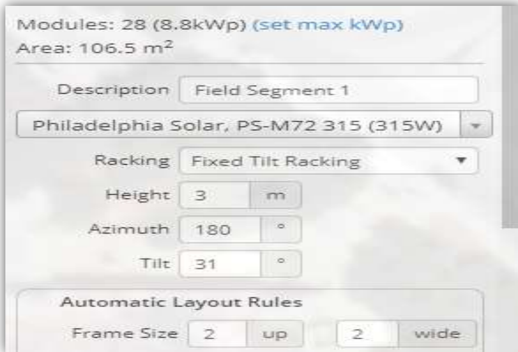
Figure 3.32 Solar System Specifications Via Helioscope Software
