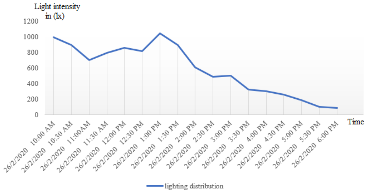
Figure 3.19 Lighting Distribution for Classroom (10) in Lux Unit
