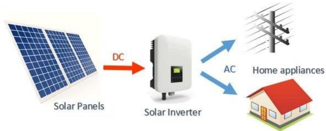
Figure 2.2: PV system components (Clean Energy Reviews 2022)
