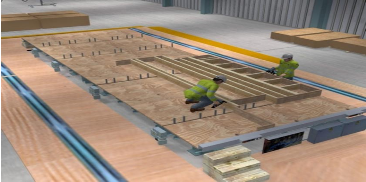
Figure 4.13: Manual Floor Framing Process
