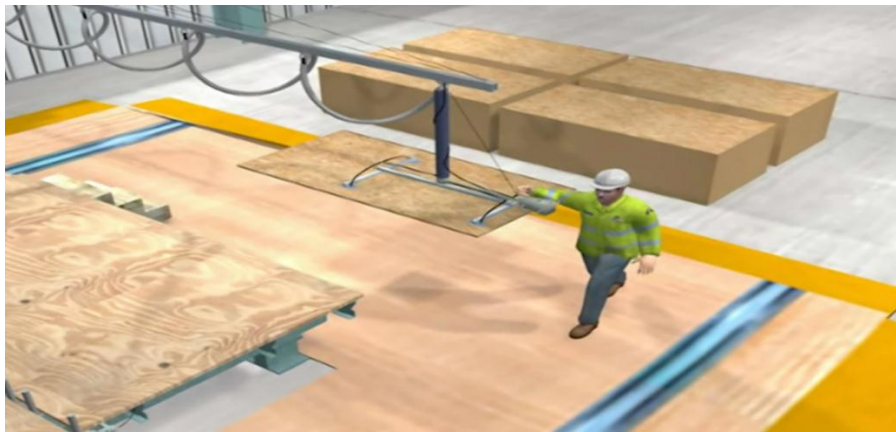
Figure 4.44: Mechanical vacuum lift system for flying in sheathing boards.
