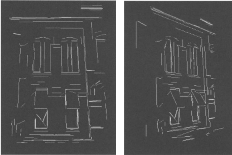
Figure 11.7 Lines extracted from the overlapping terrestrial photographs in Fig. 11.6. These 3-D vectors have been computed automatically and can now be submitted to a machine-supported manual editing and clean-up procedure.
