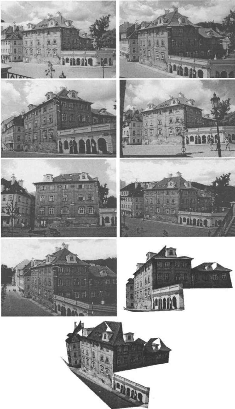
Figure 3.2 Seven input images were used to compute a projective reconstruction P . A 3D Euclidean model was then recovered by upgrading P by Pollefeys' algorithm [8].
