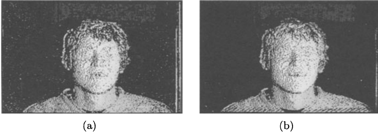
Figure 4.3 (a) Grey-encoded binocular disparity map computed for the top image pair from Fig. 4.2. Unmatched pixels are black. (b) The result of fusion of all binocular disparity maps shown in the disparity space of the same image pair.
