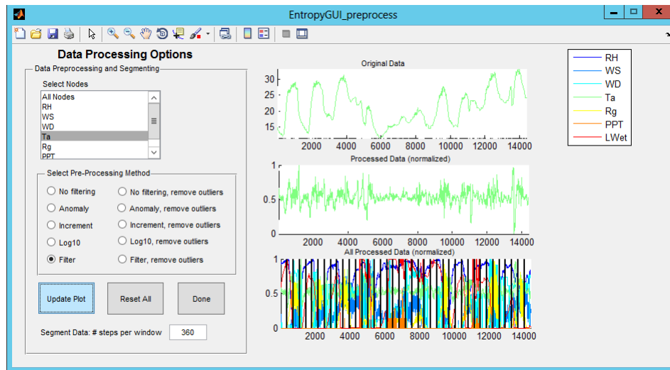
Figure B.5: TIPNet data preprocessing screen. Weather station data here has been segmented into 360 minute (6 hour) time segments as shown by black lines in bottom plot. Nodes can be pre-processed individually or as a group.
