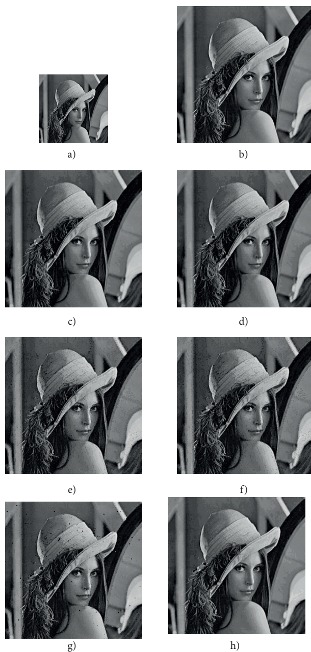
Figure 8. Lena a) original unscaled ( 256 \times 256 ) image, scaled images ( 512 \times 512 ) via ISP embedded with: b) accurate adder, c) ETA-I [6], d) ETA-II [7], e) ETA-IIM/ETA-IV [8], f) ACA [19], g) RCLA [22], and h) ProtLA.
