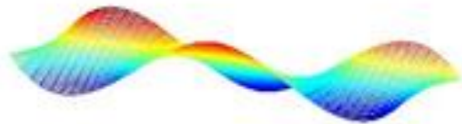
Mode 7: Third Torsion Mode (23.1 Hz)
