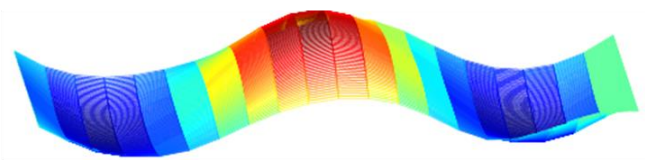
Mode 9: Third Bending Mode (40.4 Hz)
