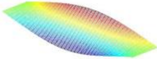
Mode 2: First Torsion Mode (6.78 Hz)
