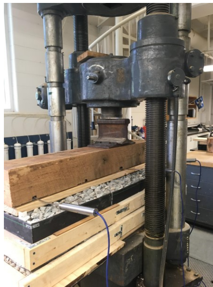
Figure 4–9 Full-scale of half-track at University of Kentucky
