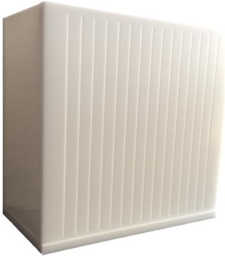
Figure 3. The ex-vivo whole lung imaging system (EWLIS). The foremost side displays the fifteen slits used to guide the physical segmentation of the lungs.
