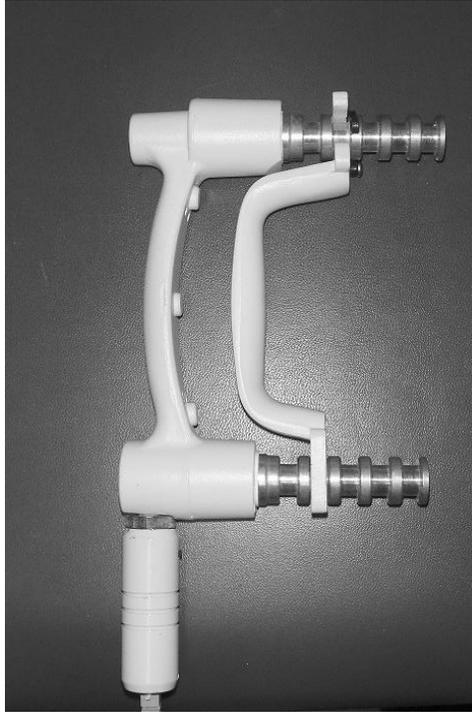
Figure 1. Modified hand grip dynamometer
