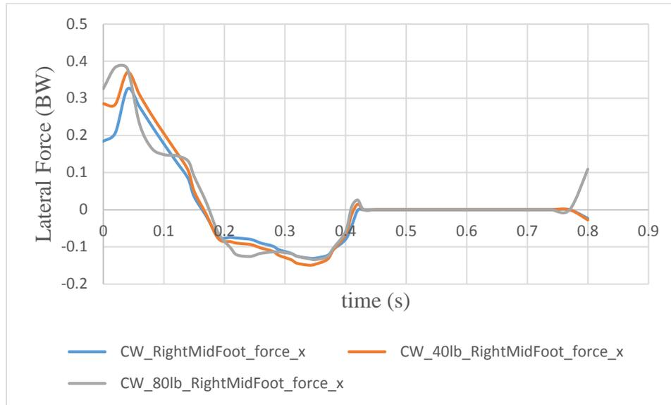
Figure 5.12: Comparison of Lateral GRF for Clock-wise Jogging Stride Simulations with No Load, 40 lb Backpack and 80 lb Backpack
