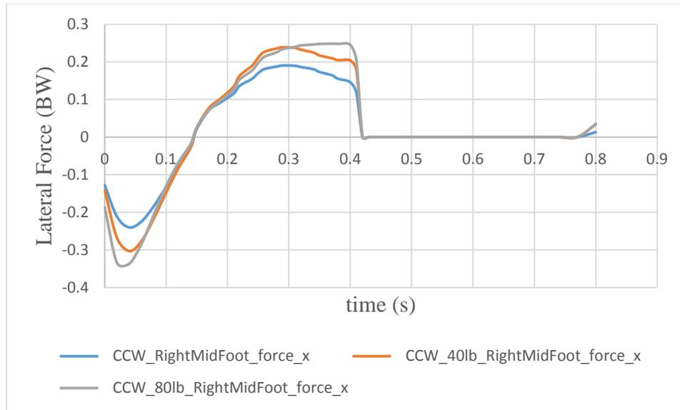
Figure 5.23: Comparison of Lateral GRF for Counter Clock-wise Jogging Stride Simulations with No Load, 40 lb Backpack and 80 lb Backpack
