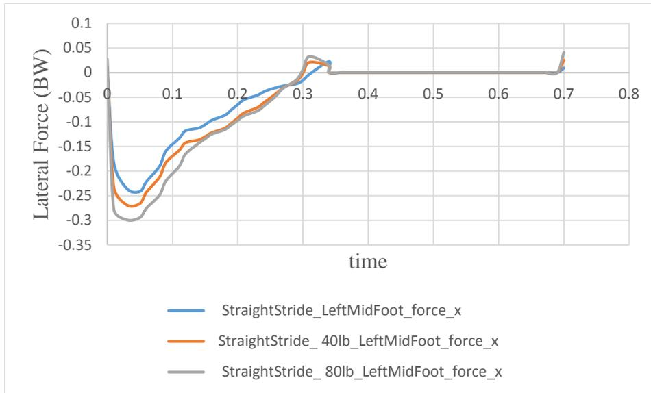
Figure 4.10 Comparison of Lateral GRF for Straight Jogging Stride Simulations with No Load, 40 lb Backpack and 80 lb Backpack
