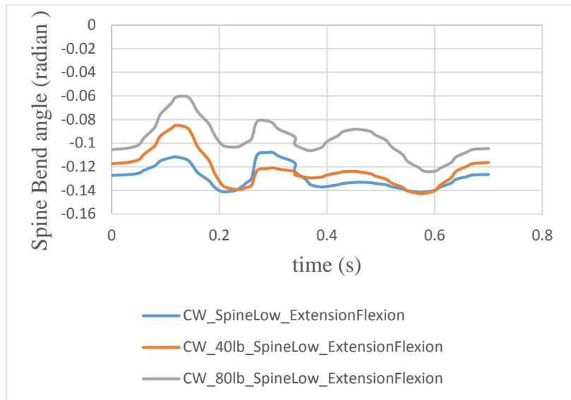
Figure 5.13: Comparison of Joint Angles for Clock-wise Jogging Stride Simulations with No Load, 40 lb Backpack and 80 lb Backpack
