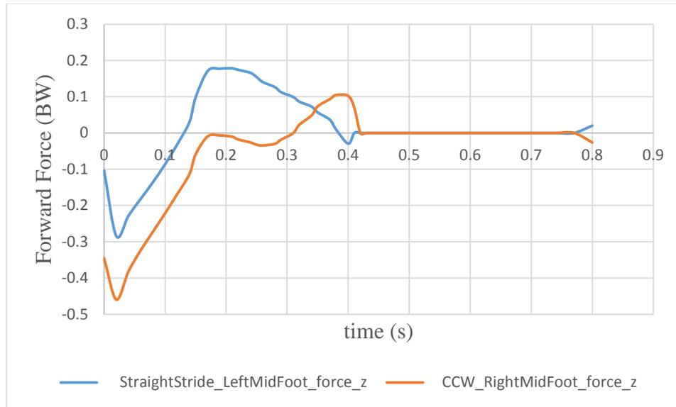
Figure 5.17: Comparison of Fore-Aft GRF for Straight Jogging Stride and Counter Clock-wise Jogging Stride Simulations
