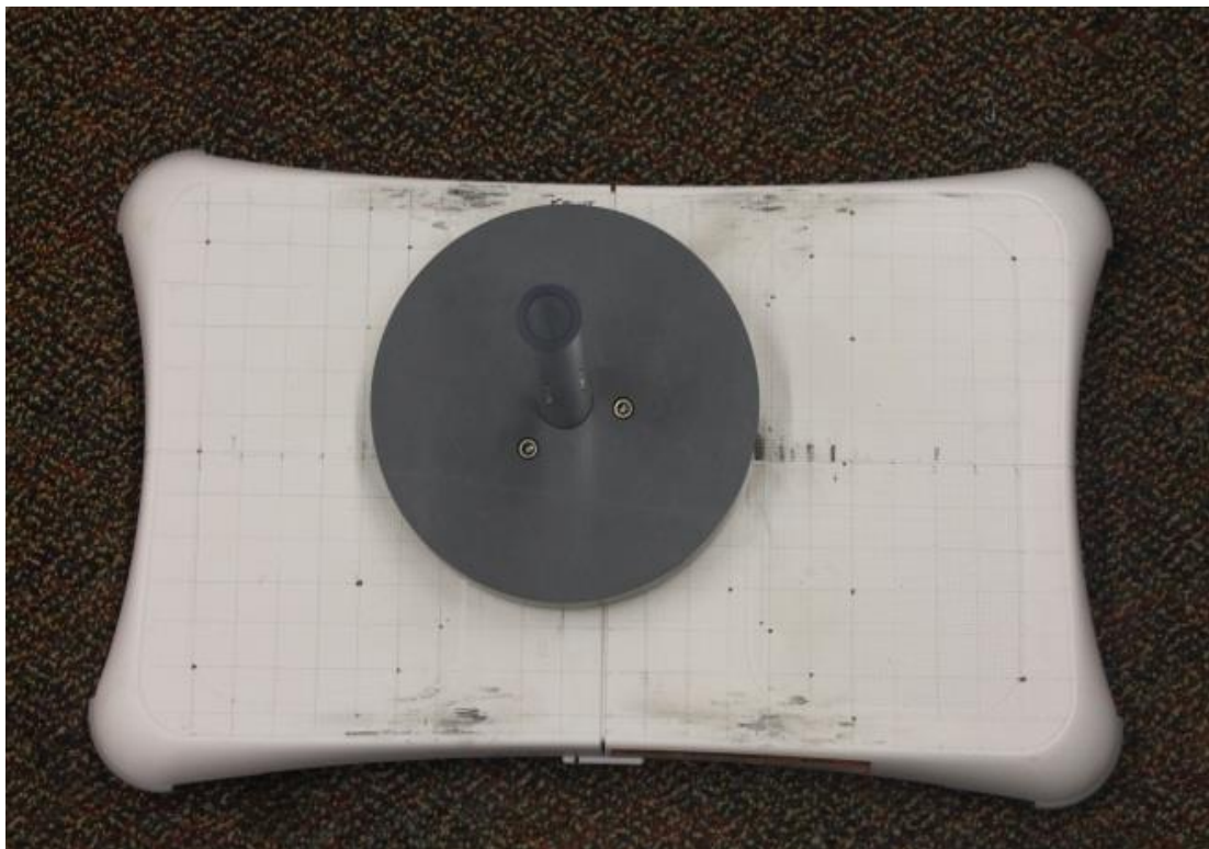
Figure 8. COP (X,Y) calibration set up
