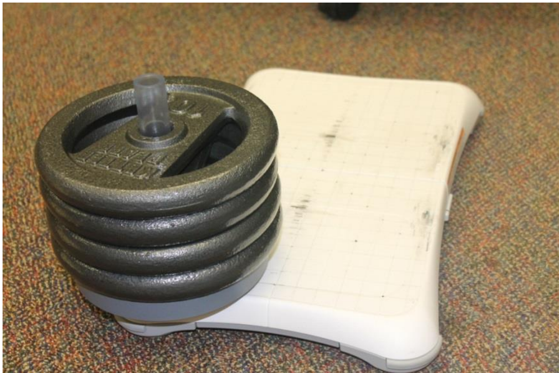
Figure 7. Calibration of ground reaction force
