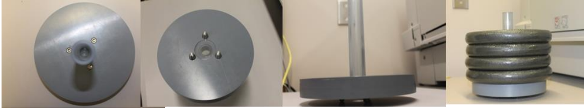
Figure 6. Point loading calibration device
