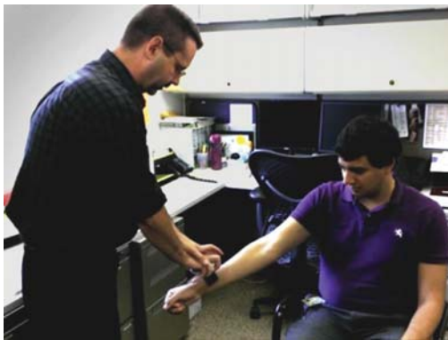
Figure 3 Example of muscle force clinical test. The subject is asked to produce maximal elevation force, and the clinical assistant restricts the motion of the subject with a MicroFet2 wireless digital handheld dynamometer. The force generated is then recorded.
