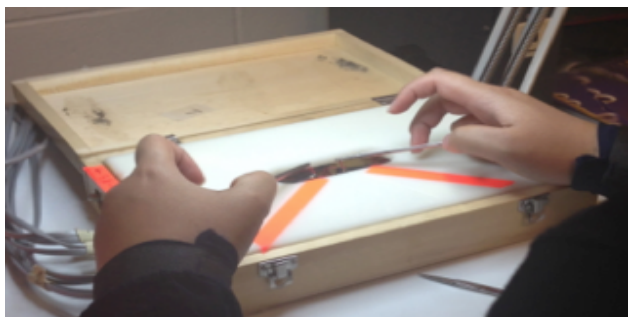
Figure 18. Velocity Transducer for tremor measurement. Orange tape guided hand/finger placement. Bimanual hemostat task (contact target/phonograph needle with stylus)
