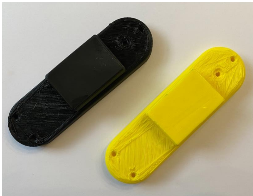
Figure 19. Printed Encasements with Uneven Print Job
