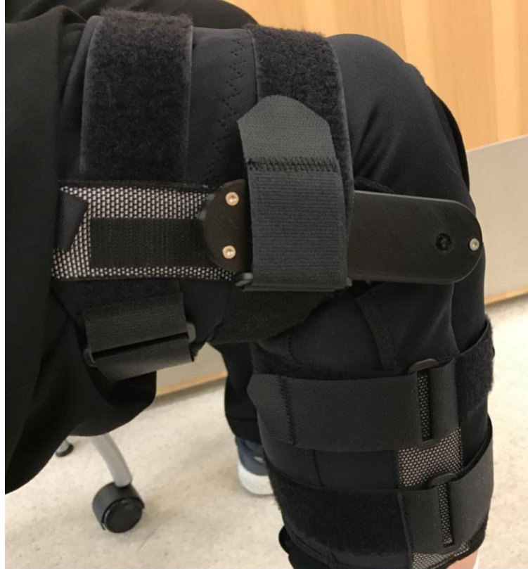
Figure 27b. The device (with the top and bottom of the casing employed) attached to the hinge system, which sits in the knee brace which is worn on a subject's leg
