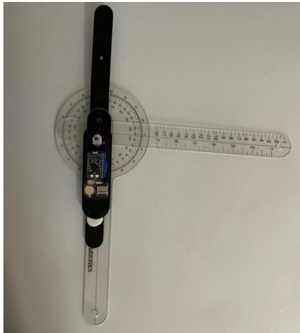
Figure 28. Starting position of the brace and device at zero degrees while the goniometer is angled at 90^\circ
