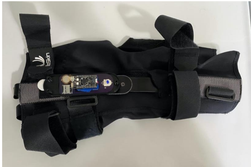
Figure 27a. Device attached to the hinge system, which sits in the knee brace
